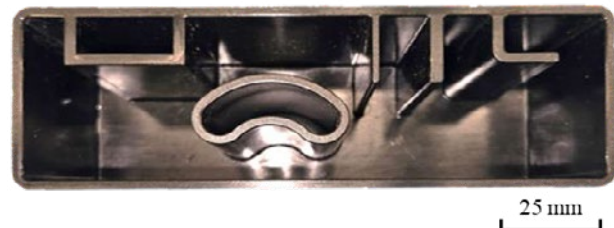
Figure 2: Injection molded component made of Makrolon 2805 with varying wall thicknesses and cavities.
