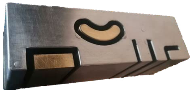
Figure 6: Assembled molding tool with optimized cores made of MM using 1.2311 and CW305G during the leakage test.
